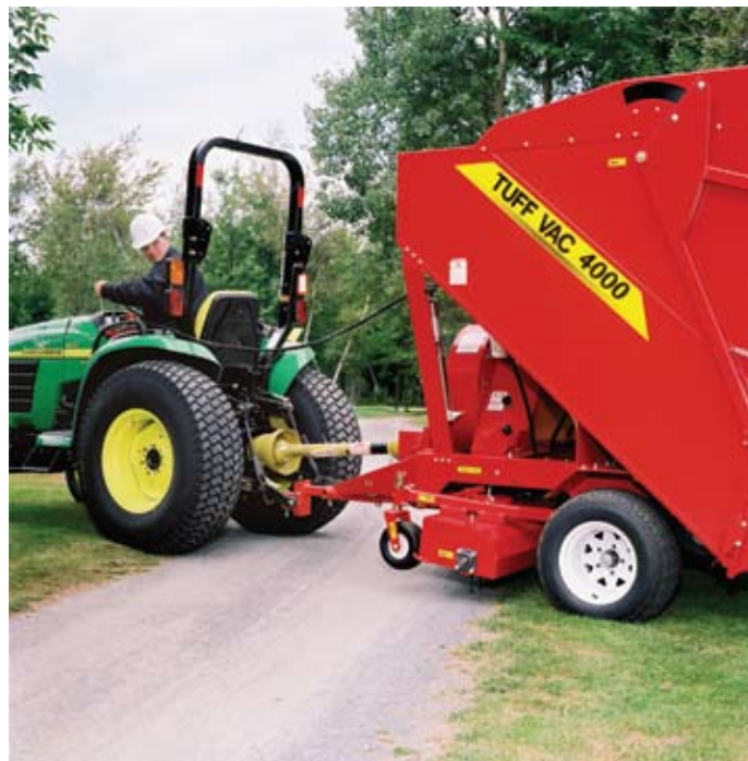
FLOATING HYDRAULIC LIFT PICKUP HEAD LETS OPERATOR CLEAR OBSTRUCTIONS FROM THE DRIVERS SEAT.
