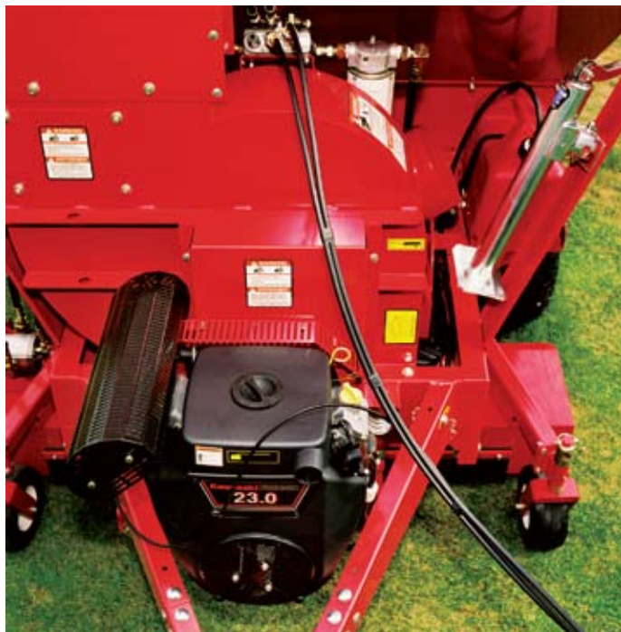
23 HP KAWASAKI ENGINE HAS EXCELLENT ACCESS FOR SERVICE. REMOVABLE GAS TANK MAKES FUELING IN REMOTE AREAS EASY.
