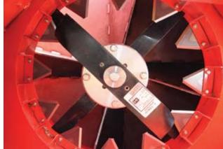
A greater holding hopper capacity with AgriMetal Multi-Vac series. The Multi-Vac series has 12 fixed knives installed just before the impeller housing, two rotary blades turning at high speed to shred leaves & branches and a third rotary blade located inside the pick-up head throat to eliminate any clogging. This exclusive internal shredder greatly increases the volume of debris that is packed into the hopper.
