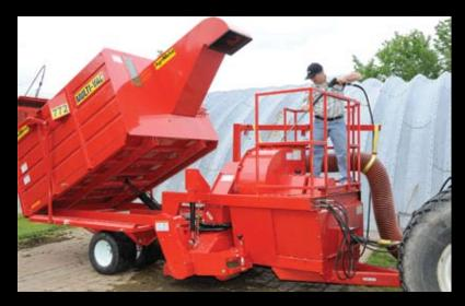
A PLATFORM LOCATED AROUND THE BLOWER HOUSING ENABLE THE OPERATOR TO SAFELY & PROPERLY CLEAN OUT THE INSIDE OF THE BLOWER. A DRAIN TRAP IS LOCATED AT THE BOTTOM OF THE BLOWER TO DRAIN WATER AND RESIDUES. ONCE THE HOPPER IS TILTED, IT IS QUICK AND EASY TO WASH OUT THE INSIDE.
