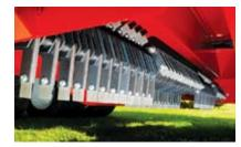
The standard vacuum head of the Multi-Vac may be replaced with a Verti-Tatch head to dethatch & pick-up debris all in one pass. (spacing 1 ½ inch cc.)
