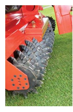
An optional slicer kit can be attached to the Verti-Tatch head. Slicer blade follow the same path as the Veticut blades for deeper penetration. (1 inch x 1 ¾ inch deep) The Verti-Tatch head equipped with a Slicer kit allow you to: de-tatch, collect & aerate fairways all in one pass. This multi purpose pick up head becomes a cost efficient investment because of its year-round use and multiple application. Only 15 minutes is required to switch pick up heads.
