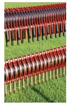
AgriMetal has developed a new brush system that is second to none in sweeping leaves and branches. The brush is made of 3/8" wide high-strength nylon fingers with shorter steel knives located between the nylon fingers. The nylon fingers and steel knives are made to freely pivot so as not to damage the turf, while throwing leaves and branches into the intake.
