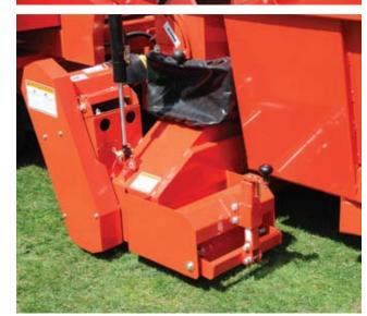
The pick-up head lowers and rises hydraulically from the operator's seat. As the operator lifts the pick-up head, the front raises first which allows to vacuum thick piles of leaves. The pickup head rides on 4 large rollers to eliminate marking, compacting and scuffing fairways.
