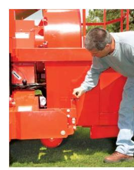
THE FRONT ROLLER HEIGHT ADJUSTMENT IS EASILY DONE WITHOUT THE NEED OF TOOLS.
